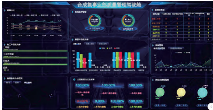
Built a high-quality cockpit of synthetic ammonia for visual presentation of key quality data and achievement of quality objectives. 搭建合成氨質量駕駛艙，實現關鍵質量數據與質量目標達成情況視覺化呈現。
